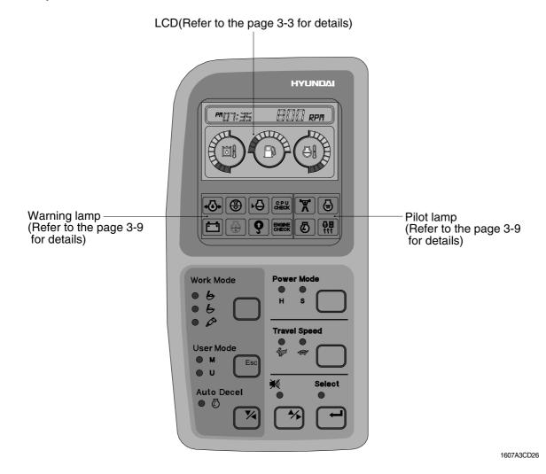
\* The warning lamp lights ON and the buzzer sounds when the machine has a problem.
