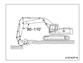
6) Operate leaving a small safety margin of cylinder stroke to prevent damage of cylinder when working with the machine.
