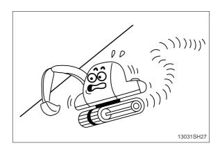
The engine angularity limits are 35 degree.
