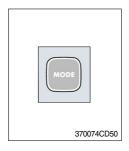
Operating this switch, it beeps and displays symbol of each mode in order.(Vent → B/L → Foot → Def → Vent)
