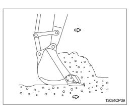
Set the tracks parallel to the line of the ditch to be excavated when digging ditch. Do not swing while digging.
