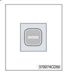
Operating this switch, it beeps and displays symbol of each mode in order.(Vent → B/L → Foot → Def → Vent)
