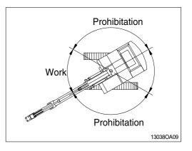
8) TAKE CARE OF CHISEL AND BOOM INTERFACE Make sure of the arm and bucket control lever operation.
