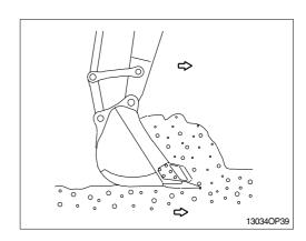
4) Set the tracks parallel to the line of the ditch to be excavated when digging ditch. Do not swing while digging.
