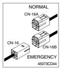
(1) When the CAN communication between the ECM and the MCU controller is abnormal due to malfunction of the MCU controller, change CN-16 connection from CN-16A to CN-16B and then control the engine speed by rotating accel dial switch.
