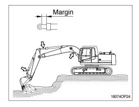
Keep the bucket to the dumping position and the arm horizontal when dumping the soil from the bucket.
