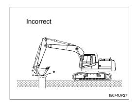
10) Do not use the bucket to crack hard objects like concrete or rocks.
