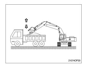
8) Operate stop of swing considering the swing slip distance is created by inertia after neutralizing the swing lever.
