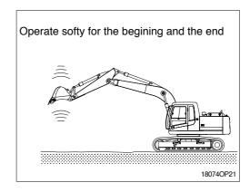
The digging resistance and wearing of tooth can be reduced by putting the end of bucket tooth to the digging direction.
