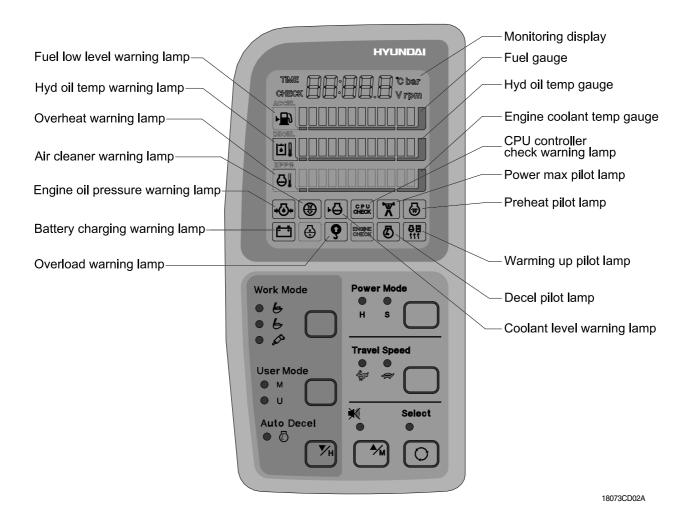
\* The warming lamp lights ON and the buzzer sounds when the machine has a problem.
