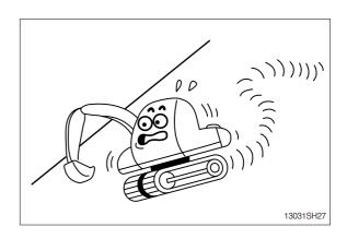
The engine angularity limits are 35 degree. Do not operate by more than the engine limits in any case.
