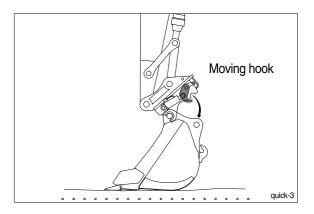
(5) Press quick clamp switch to lock position.
