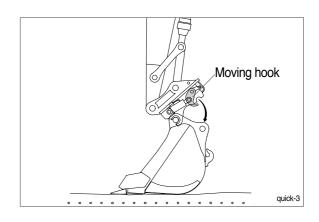
(5) Press quick clamp switch to lock position. Operate RCV lever to bucket-in position. Be sure to check connection status between bucket pins and hooks of quick clamp
