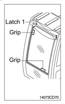
(1) Perform the following procedure in order to open the upper windshield. Release both latches(1) in order to release the upper windshield. Hold both grips that are located at the bottom of the windshield frame and at the top of the windshield frame push the windshield upward.
