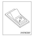
(1) This switch is used to select breaker.The breaker operates only when this switch is selected.
