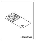
(1) This switch is used to turns ON the cab light on the cab.
