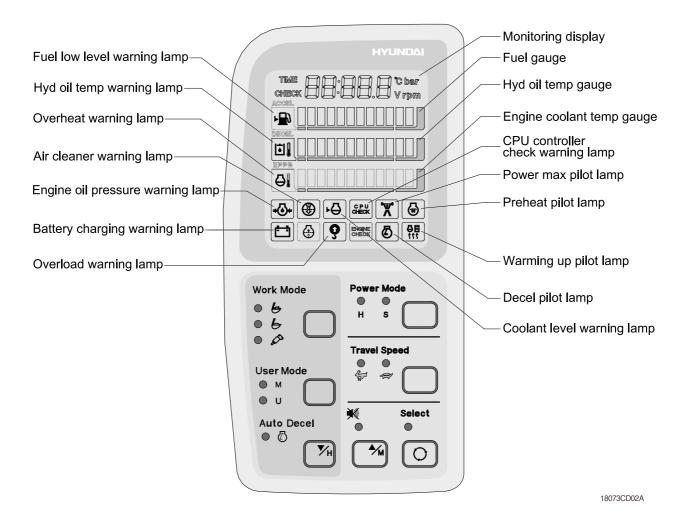
The warming lamp lights ON and the buzzer sounds when the machine has a problem. In this case, press the buzzer stop switch and buzzer stop, but the warming lamp lights until the problem is cleared.
