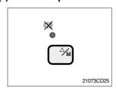
When the starting switch is turned ON first, normally the alarm buzzer sounds for 2 seconds during lamp check operation.
