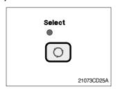
This switch is used to select the monitor display function.
