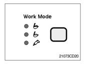
This switch is to select the machine operation mode, which shifts from general operation mode to heavy operation mode and breaker mode in a raw by pressing the switch.
