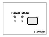
The lamp of selected mode is turned ON by pressing the switch( ).
