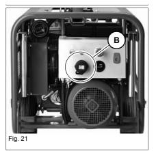
• Accessories outlet **B** (7.5 kW version): supplies the battery charger with electric power, for example.
