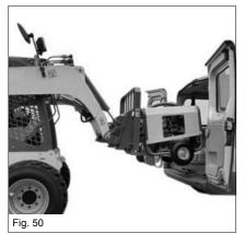
The power unit can also be loaded with a fork lift truck or construction machine with pallet forks.
