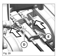
14.Connect the hydraulic hose connection **D** to the excavator.15.Connect the hydraulic hose connection **E** to the excavator.
