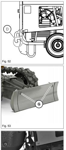
1. Hitch the stabilizer blade hooks **D** in transport holes **G** to ensure a safe hold of the power unit.
