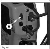
Connect the 12 V connector **A** to the 12 V outlet **B**.
