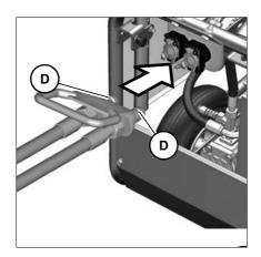
13.Connect the hydraulic hose connections **D** to the power unit.
