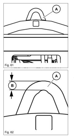
Do not perform any crane-lifting if the material thickness  ${\bf B}$  of lifting point  ${\bf A}$  is less than 23 mm (0.9 in).
