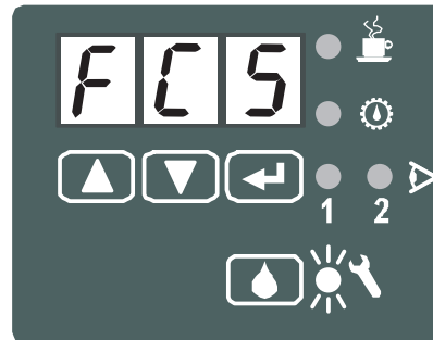
Figure 167 Device display-Three-digit LED display
