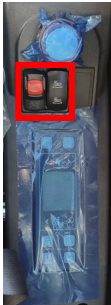
Elevating cab switch
