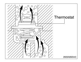
③ Install the cap. Operate the engine until it reaches a temperature 80°C (176°F), and check for coolant leaks. Check the coolant level again to make sure the system is full of coolant.
