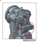
(1) The TCU uses sensors from the transmission, gear selector lever, as well as data provided by the ECU to calculate how and when to change gears.
