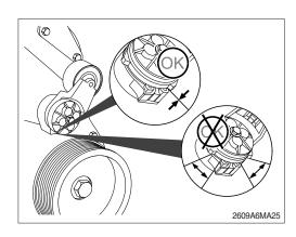
(4) Check the location of the drive belt on the belt tensioner pulley. The belt should be centered on, or close to the middle of, the pulley. Misaligned belts, either too far forward or backward, can cause belt wear, belt roll-offs, or increase uneven tensioner bushing wear.
