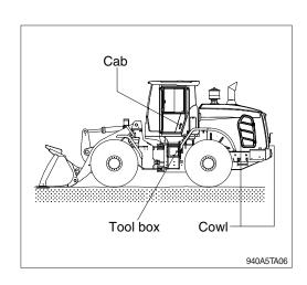
6) Block the tires and fix firmly with wire rope or chain to prevent the machine from moving during transportation.
