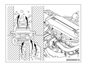
② Operate the engine for 5 minutes with the coolant temperature above 80°C (176°F). Shut the engine off, and drain the cooling system.
