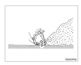
If the machine operates with the front tires lifted, tractive effort will be reduced significantly and excessive force will be applied to the rear tires. Avoid operating in this manner.
