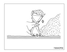
③ If material is dense, move the bucket control lever left and right to move the bucket teeth up and down to loosen the pile.
