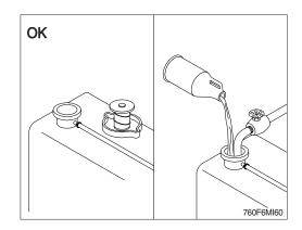
During filling, air must be vented from the engine coolant passages. The system must be filled slowly to prevent air locks. Wait 2 to 3 minutes to allow air to be vented, then add mixture to bring the level to the top.
