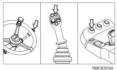
(1) Depressing the horn button(s) will engage the horn.
