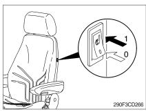
① The seat heater can be turned on/off by pressing the switch.
