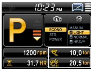
The example of the weighing system
